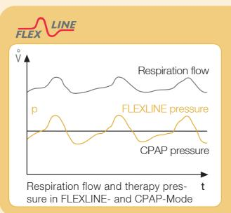
In the FLEXLINE mode the pressure adjusts proportionally to the individual respiration flow. This means an increase in pressure on inspiration and a reduction in pressure on expiration. This results in a particularly gentle therapy.
